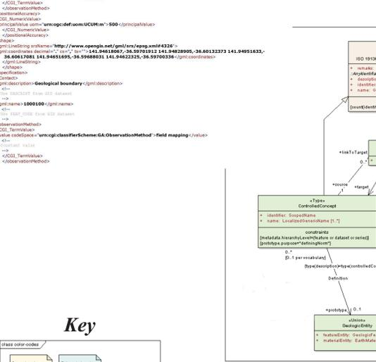
The model incorporates a structure for controlled concepts which can be defined in terms of normative descriptions of geologic units or earth materials. These can be built into Vocabularies, such as stratigraphic lexicons.
